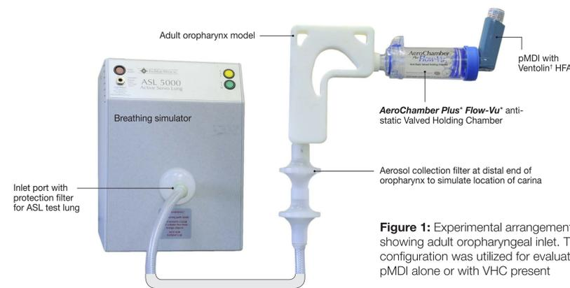
**Figure 1:** Experimental arrangement showing adult oropharyngeal inlet. The same configuration was utilized for evaluation of pMDI alone or with VHC present
