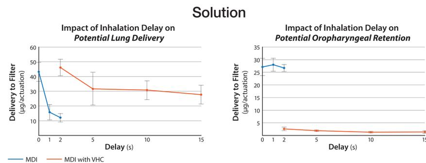
**Figure 3:** Effect of Inhalation Delay on BDP Solution-Formulated pMDI-Delivery on Mass of Medication Recovered from (A) Distal Filter of the ADAM Model and (B) the Oropharyngeal Airway
