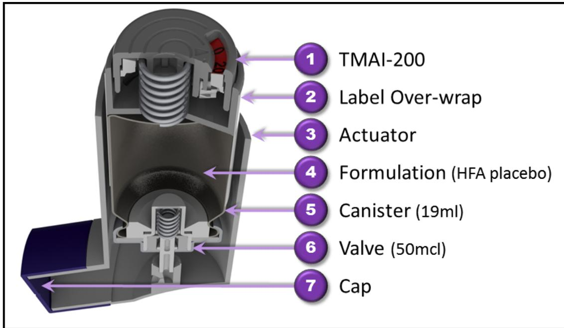
**Figure 1: Schematic of TMAI-200 Dose Indicator Integrated with a Pressurized Metered Dose Inhaler**
