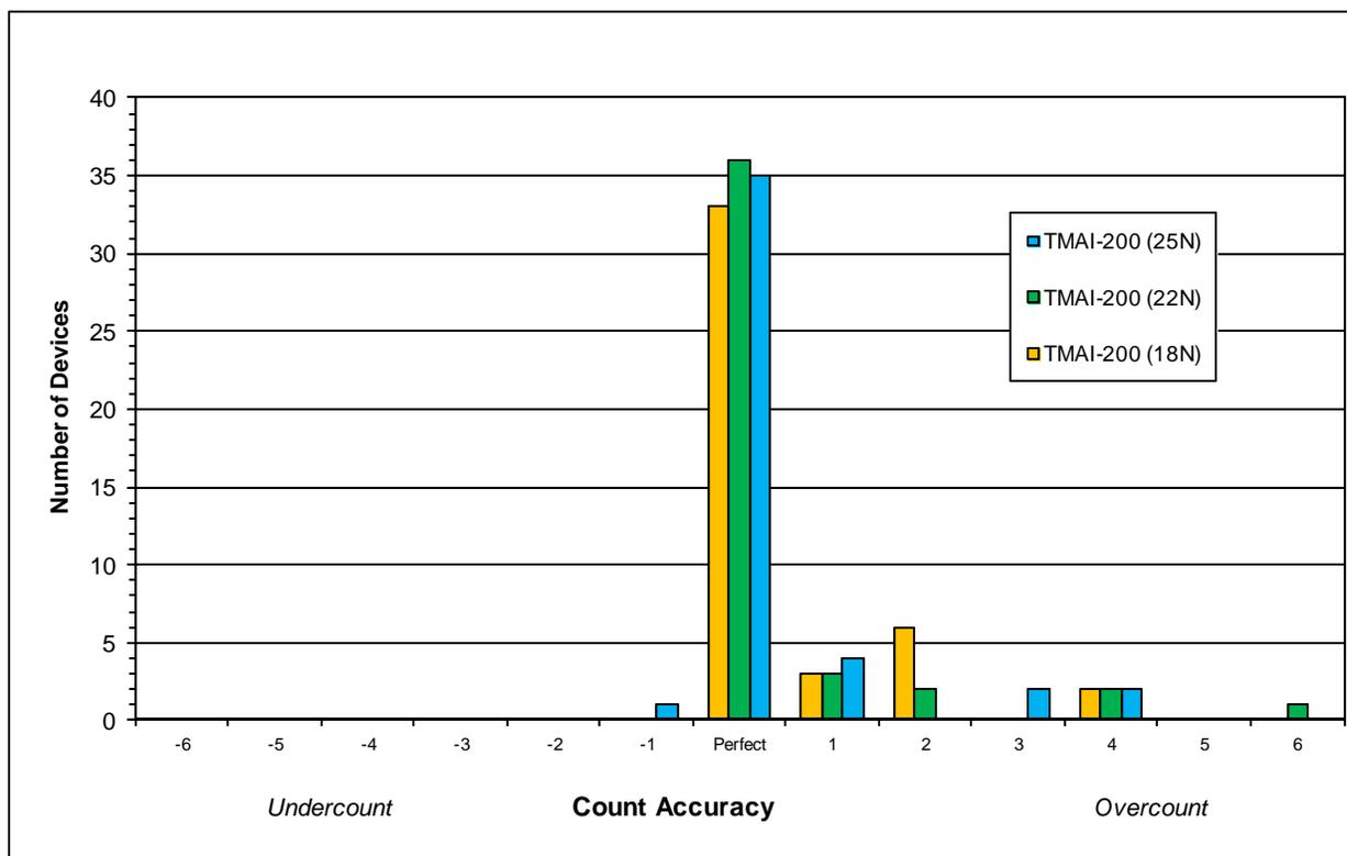
**Figure 2: Counting Accuracy for Three FTC Options of the TMAI-200 Dose Indicator Based on Device Number**
