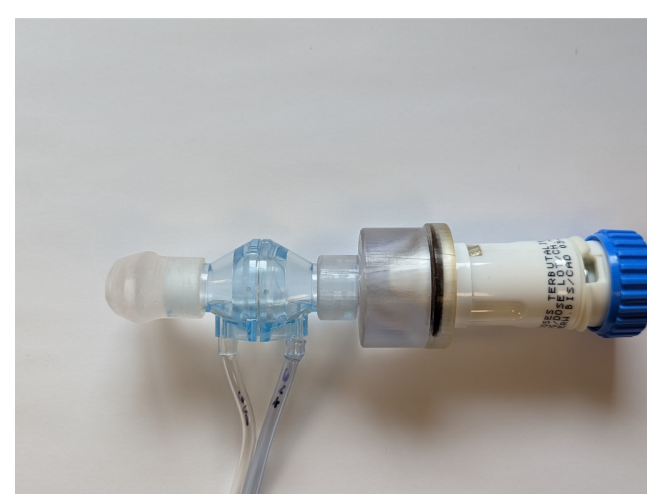
Figure 3: Turbuhaler* DPI with flow sensor/adaptor
