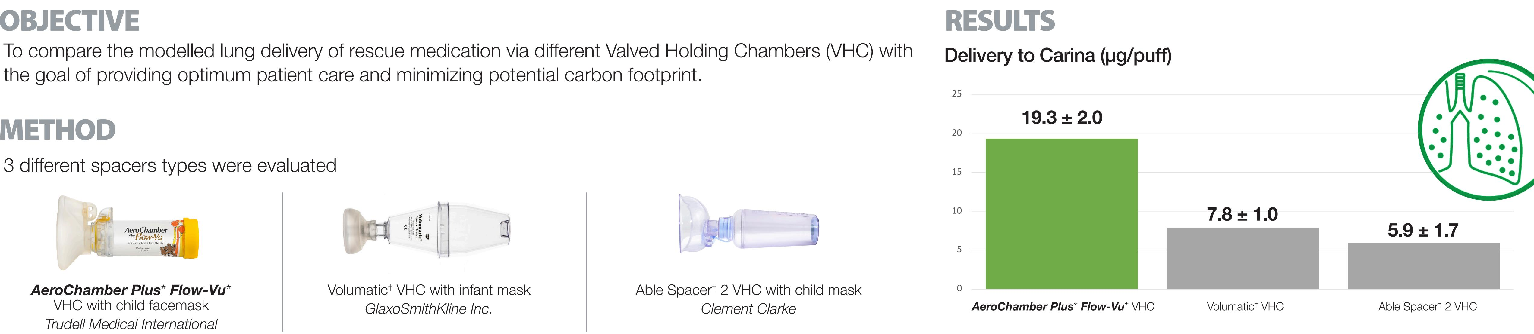
Breathing Simulator evaluation; Tidal volume=155-mL, I:E ratio=1:2, rate=25 cycles/min.
